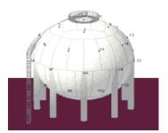
Similar to the Tank testing sensors are mounted on the sphere or vessel at calculated locations and load/pressure is applied during the data collection to record for acoustic emissions that comes from active anomalies. The mechanisms that can give rise to acoustic emission in are: fatigue crack nucleation and growth, plastic deformation, creep, fracture and decohesion of inclusions, stress corrosion cracking, hydrogen embrittlement, corrosion fatigue and others.
