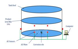
The tank bottom floor is a crucial component of large oil storage tanks, and its status has a pivotal impact on the integrity of the entire tank. Tank Bottom being in-accessible to inspect under service, Acoustic Emission (AE) monitoring has become internationally recognized on-intrusive method to be capable of assessing the tank bottom floor without the necessity of prior tank cleaning.
